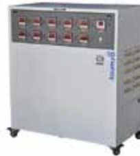
Hydrostatic Pressure Test
